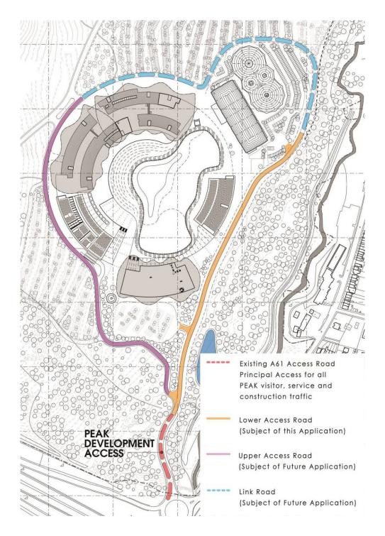
4.3 The lower access road provides 3 No radii access spurs along its length. The first connects to the intended upper access road which is to run north through semi-improved grassland towards the Peak development area. The second access spur connects to the intended Gateway building and car park area. The road continues around the development area along the base of the sloping land
