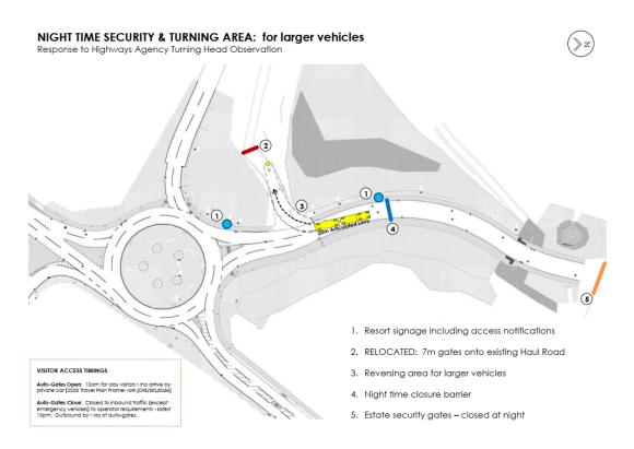
There is insufficient space within highway limits to provide a formal turning head on the adopted spur from the roundabout and the HA did not consider this was necessary when designing the scheme however the opportunities to turn exist as shown in the diagrams above and will ensure that no vehicle has to reverse out onto the traffic roundabout.
